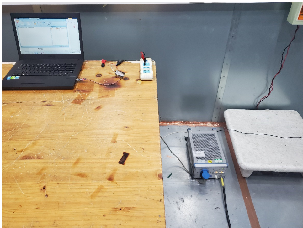
Picture 2 Conducted Emission Test Setup
