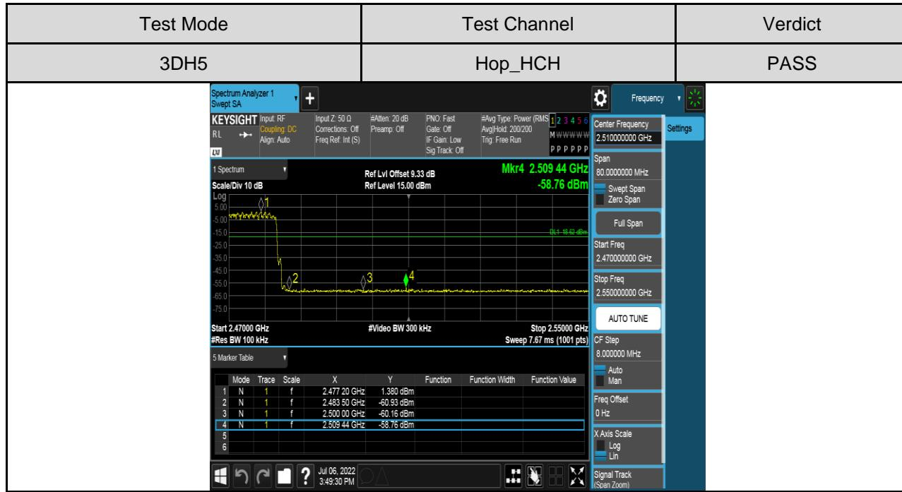
**PART 3: CONDUCTED SPURIOUS EMISSION****TEST RESULTS TABLE**
