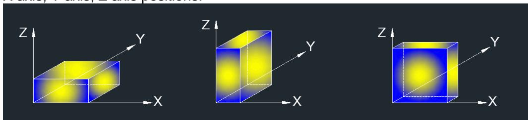
Note: For all radiated test, EUT in each of three orthogonal axis emissions had been tested, but only the worse case (X axis) data recorded in the report.
