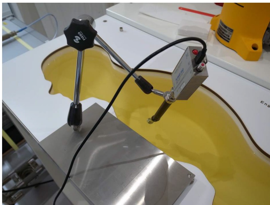
(b) Example Photo: Dielectric Parameter Measurement
