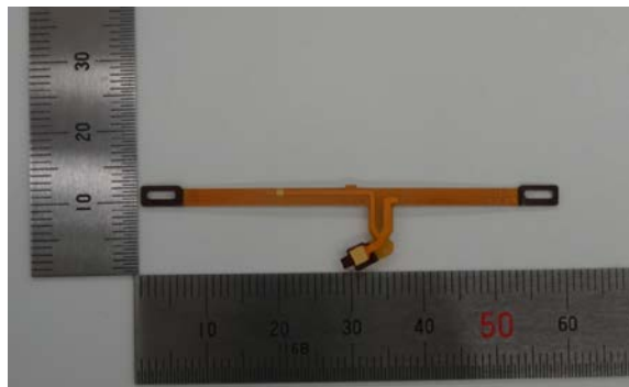
WiFi Antenna (FPC-2023) in normal shape (not folded)
