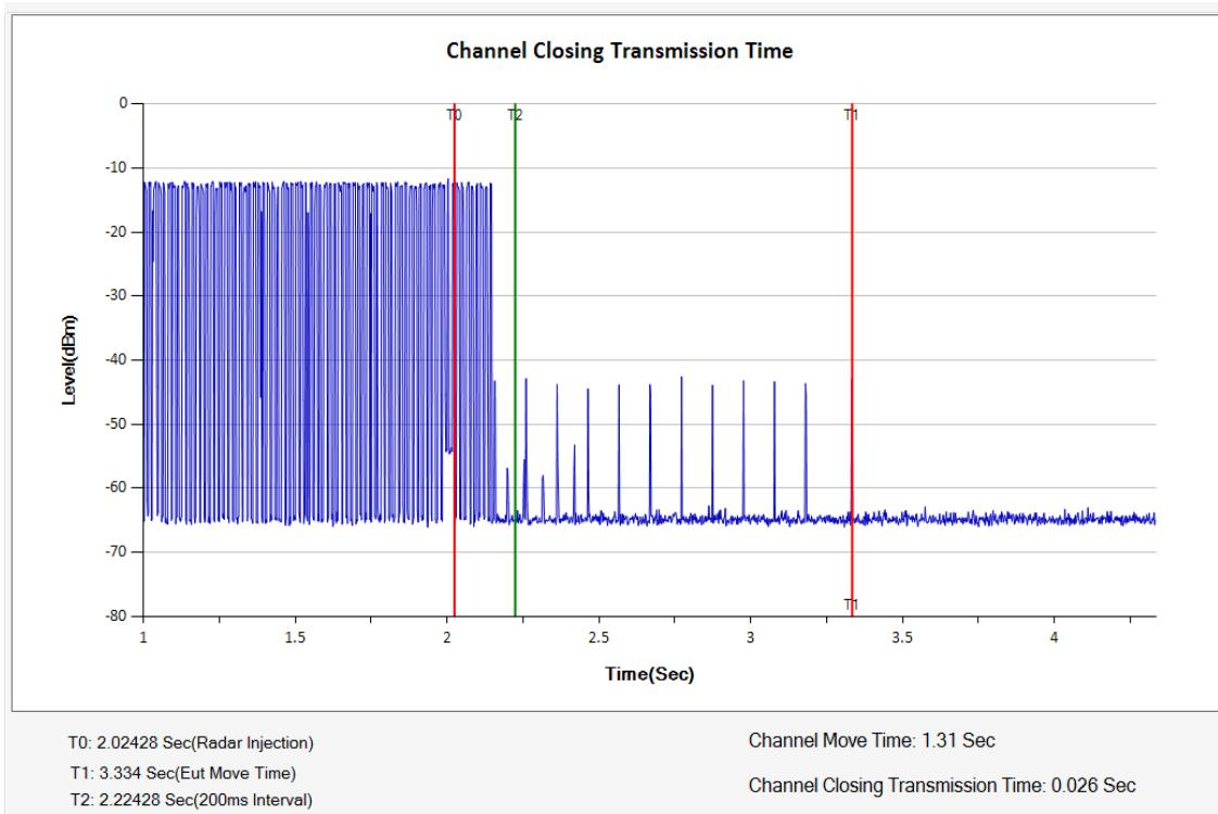
**Verdict:** Note: narrowing the sweep time as the good engineering process for the verification of transmission closing in 200ms
