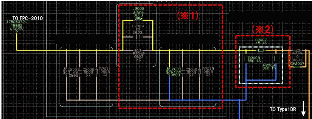
(※1) L2002/L2003 are used for RF antenna matching adjustment. It is not used for controlling antenna characteristics.
