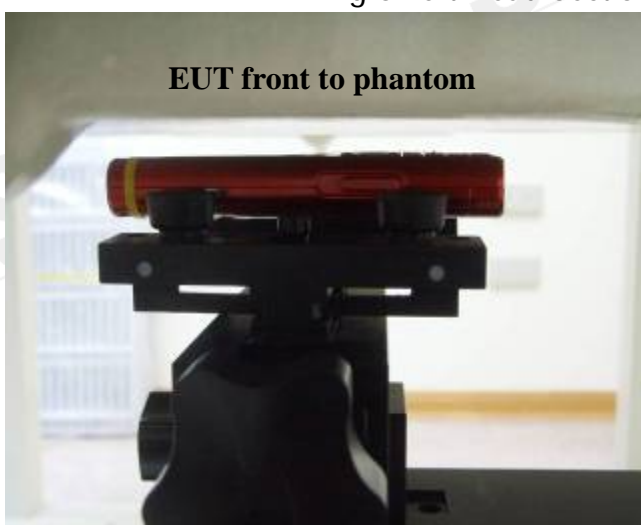
Fig.7 Body worn- EUT front to flat phantom and distance between flat phantom and mobile phone is 1.5 cm
