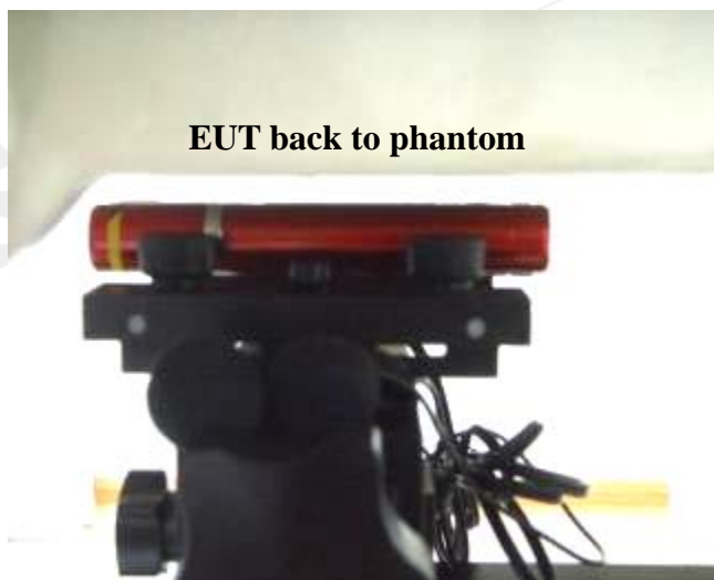
Fig.9 Body worn- EUT back to flat phantom with headset and distance between flat phantom and mobile phone is 1.5 cm
