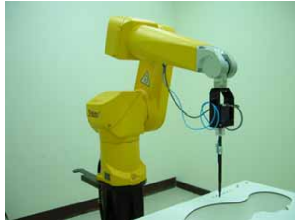
Fig. 5.2 Probe Setup on Robot
