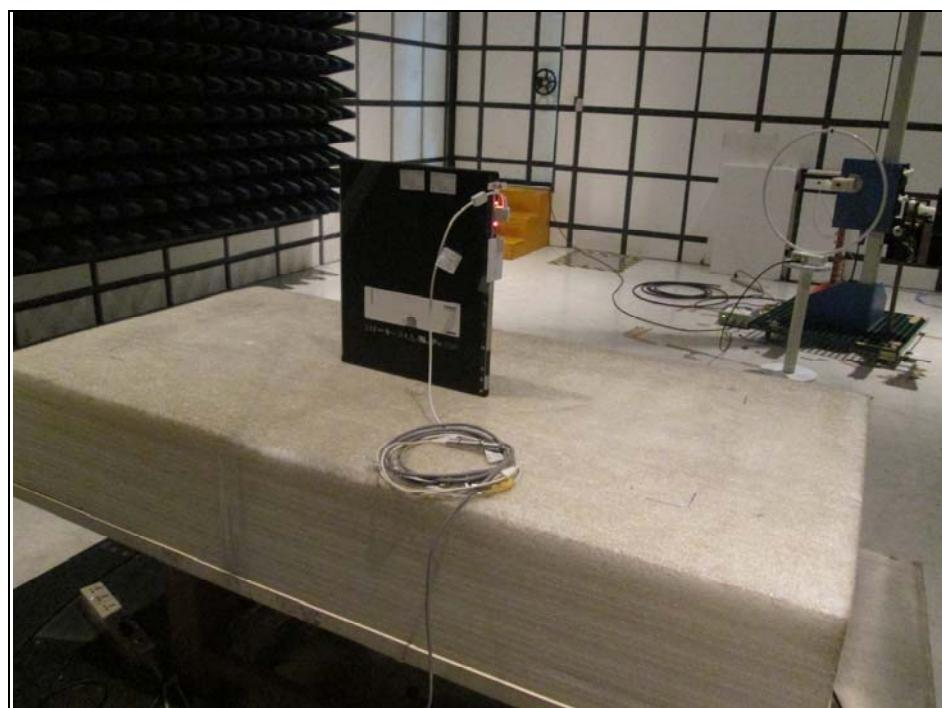
Radiated Emission Test (Frequency range 30MHz to 1GHz)
