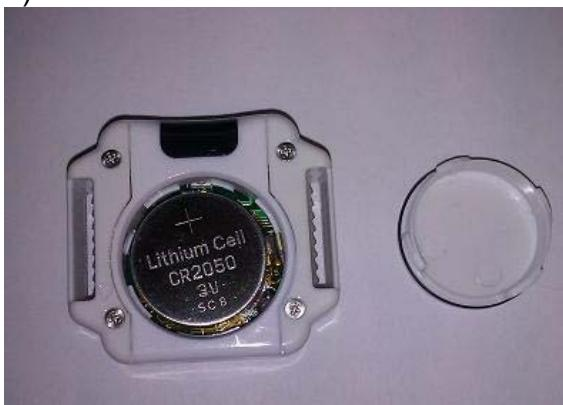
Place the coin-cell battery with positive terminal (+) face outwards.
