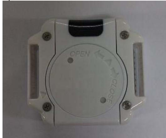
After tighten up the cover, it should be flush with the casing (body).
