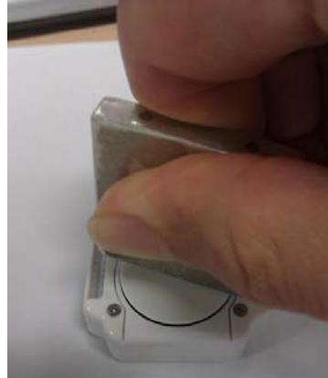
Press a little bit and turning clockwise for tightening. (*Approximately 10 degree, there is a stopper so won't overturn*).
