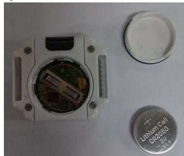
Prepare a CR2050 coin cell battery and a battery cover as shown above
