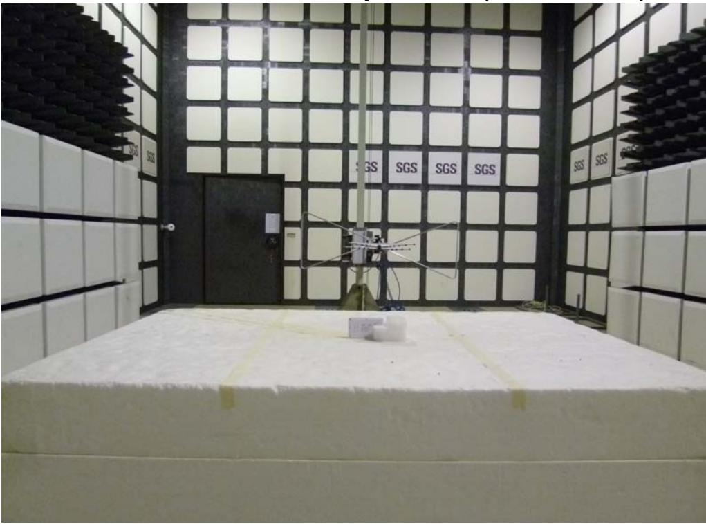
**Radiated Emission Set up Photos (Above 1GHz)**
