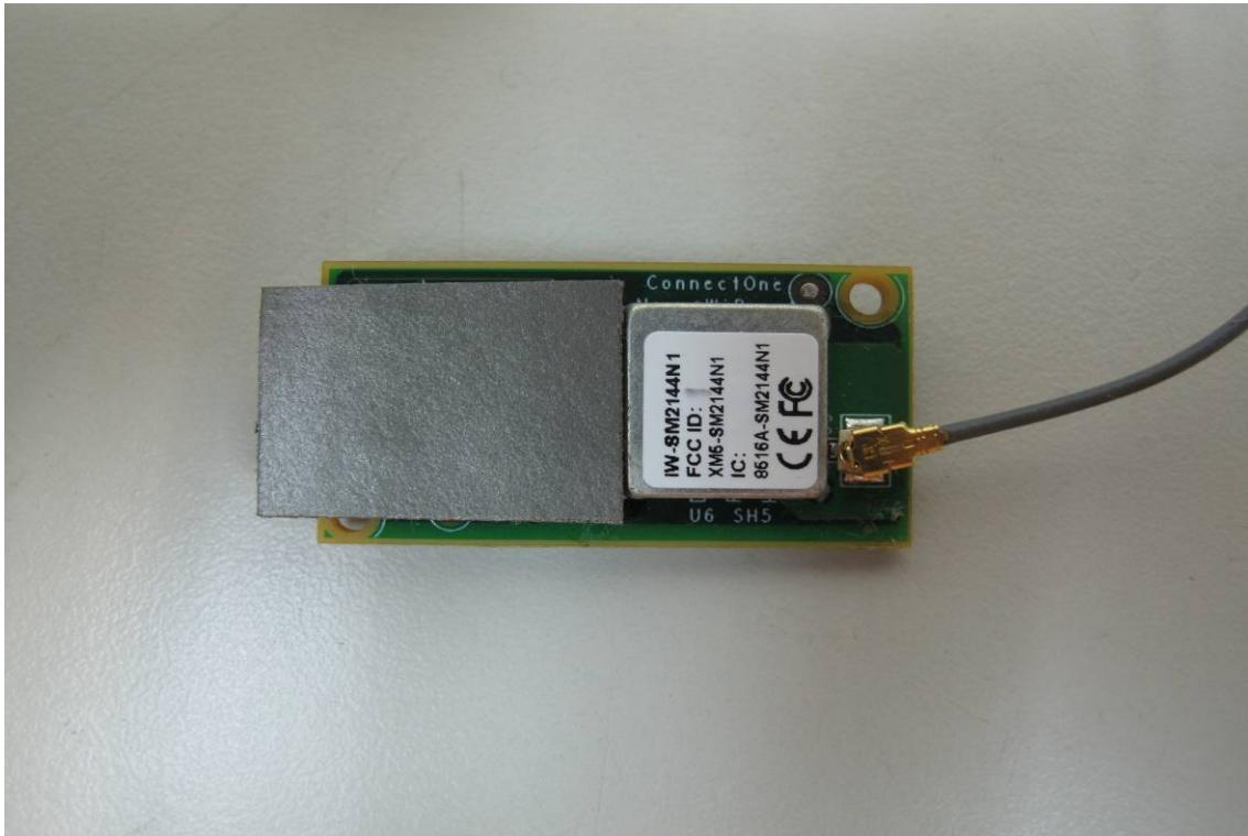
*Internal View of EUT - 12(WLAN Module)*
