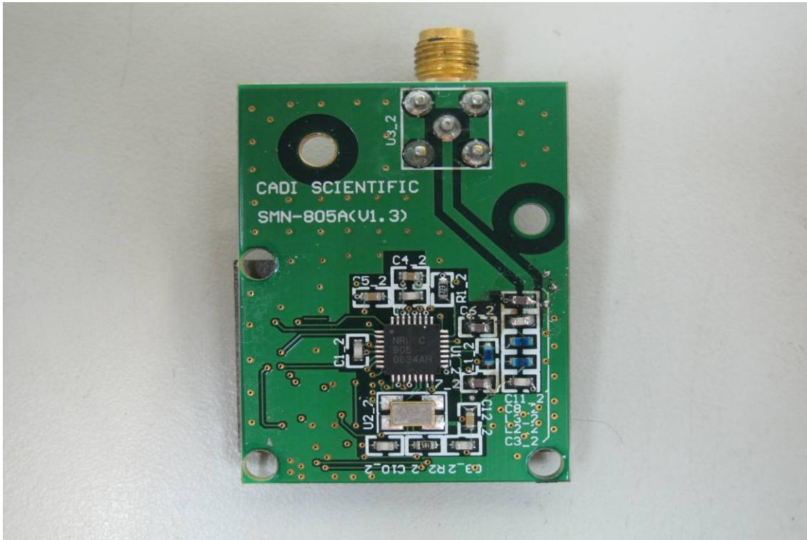
*Internal View of EUT - 10 (Wireless Module)*
