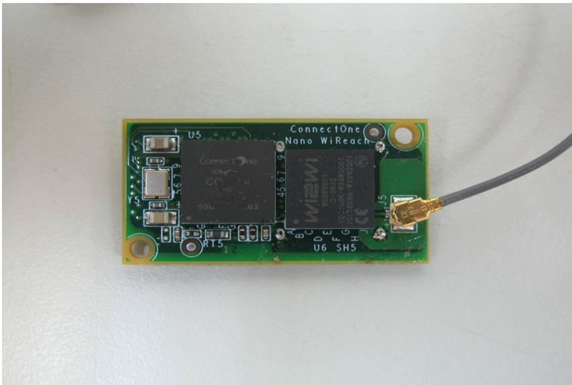
*Internal View of EUT – 14 (WLAN Module)*
