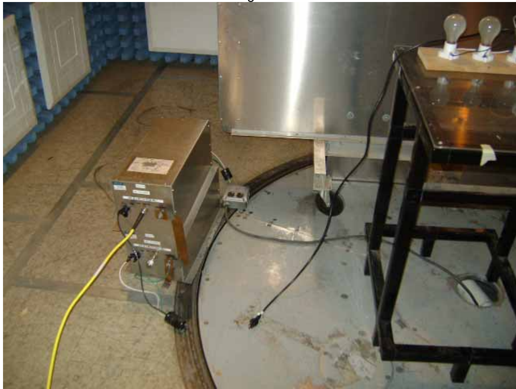
Test Setup for Conducted Emissions
