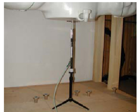
Figure 12.1 Dipole Validation Test Setup
