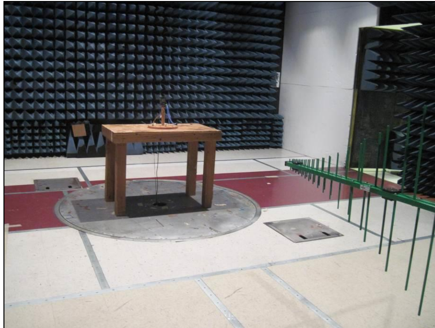
Photograph 2. Radiated Spurious Emissions, 30 MHz – 18 GHz, Test Setup
