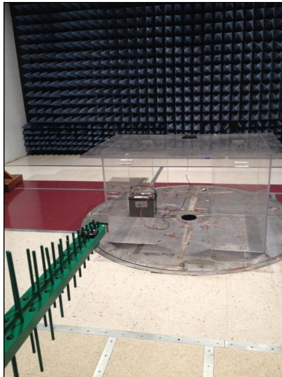
Photograph 2. Radiated Emissions, Test Setup, 30 MHz – 1 GHz
