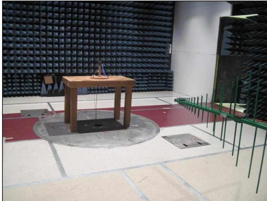
Photograph 4. Radiated Spurious Emissions, 30 MHz – 18 GHz, Test Setup
