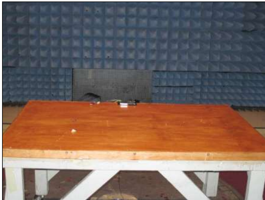
Photograph 3. Radiated Emission, Test Setup
