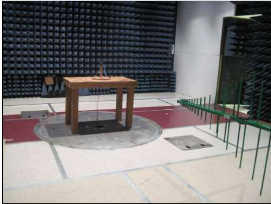
Photograph 4. Radiated Spurious Emissions 30 MHz – 1 GHz, Test Setup
