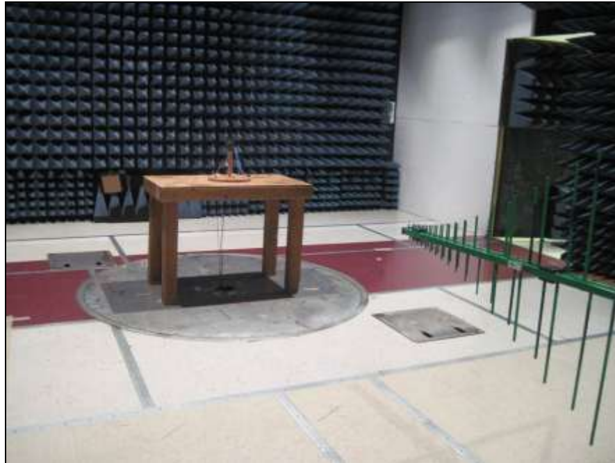
Photograph 4. Radiated Spurious Emissions, 30 MHz – 18 GHz, Test Setup
