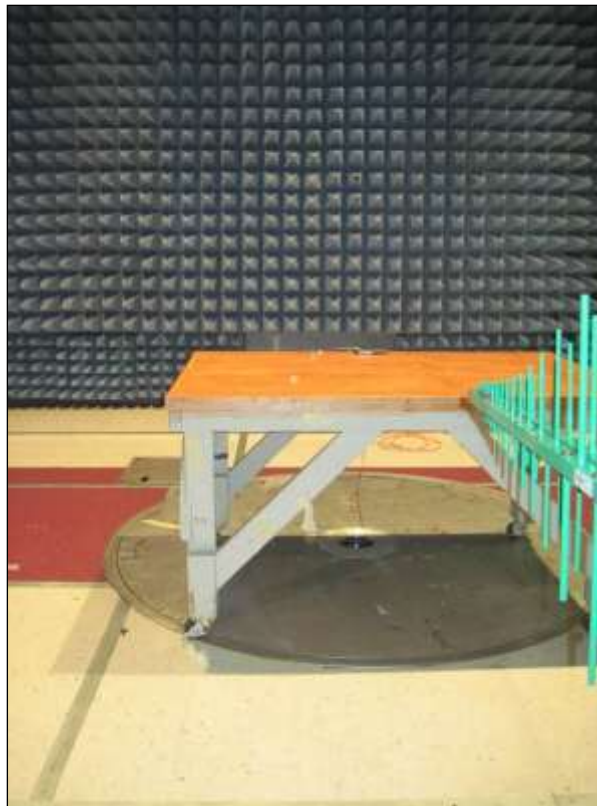
Photograph 2. Radiated Emissions, Test Setup, Antenna View
