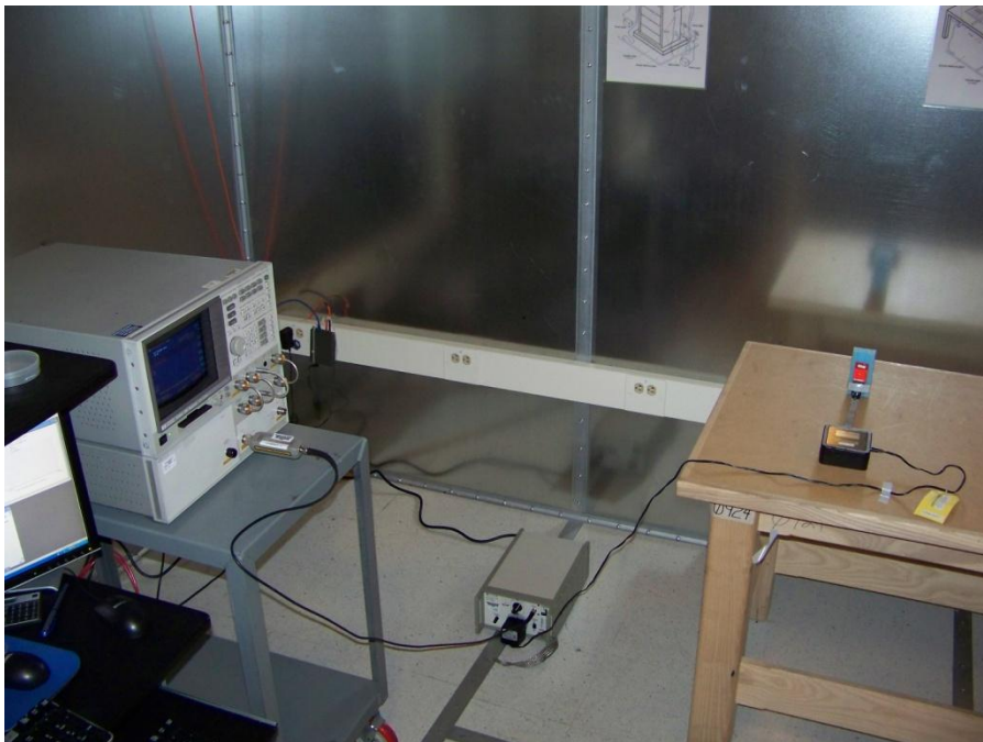
Figure 17: Equipment setup during Conducted RF Emissions tests – representative test showing EUT (Tx-LMA mode) powered by a wall-type step-down transformer.
