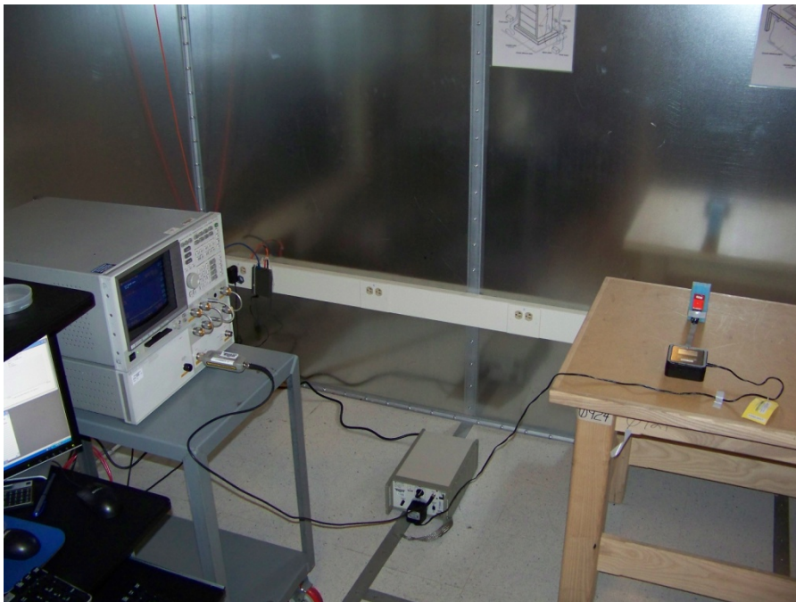
Figure 44: Equipment setup during Conducted RF Emissions tests – representative test showing EUT (Tx-LMA mode) powered by a wall-type step-down transformer.
