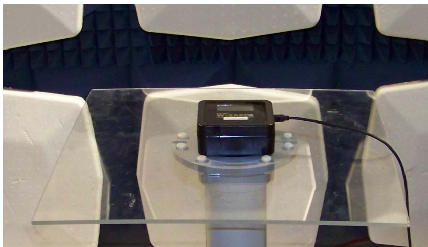
Figure 10: Horizontal orientation reference point- tests for host qualification.
