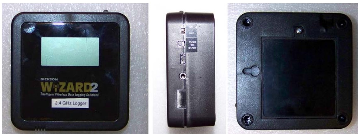
Figure 1: The Dickson 'Wizard2' telemetry system, as tested: Front view, right side view, and rear view.
