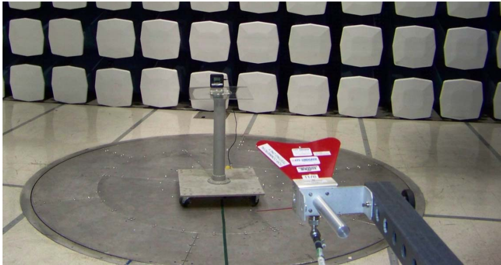
Figure 59: EUT on Test Pedestal during Occupied Bandwidth testing.
