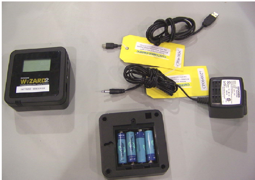
Figure 3: Power source options of Battery, USB, and Wall-type Step-Down transformer may be used with the WiZARD2.
