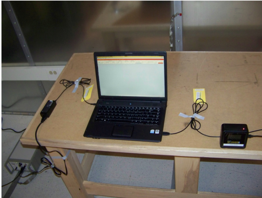
Figure 43: Equipment setup during Conducted RF Emissions tests – representative test showing EUT powered through USB port of a lap-top computer.
