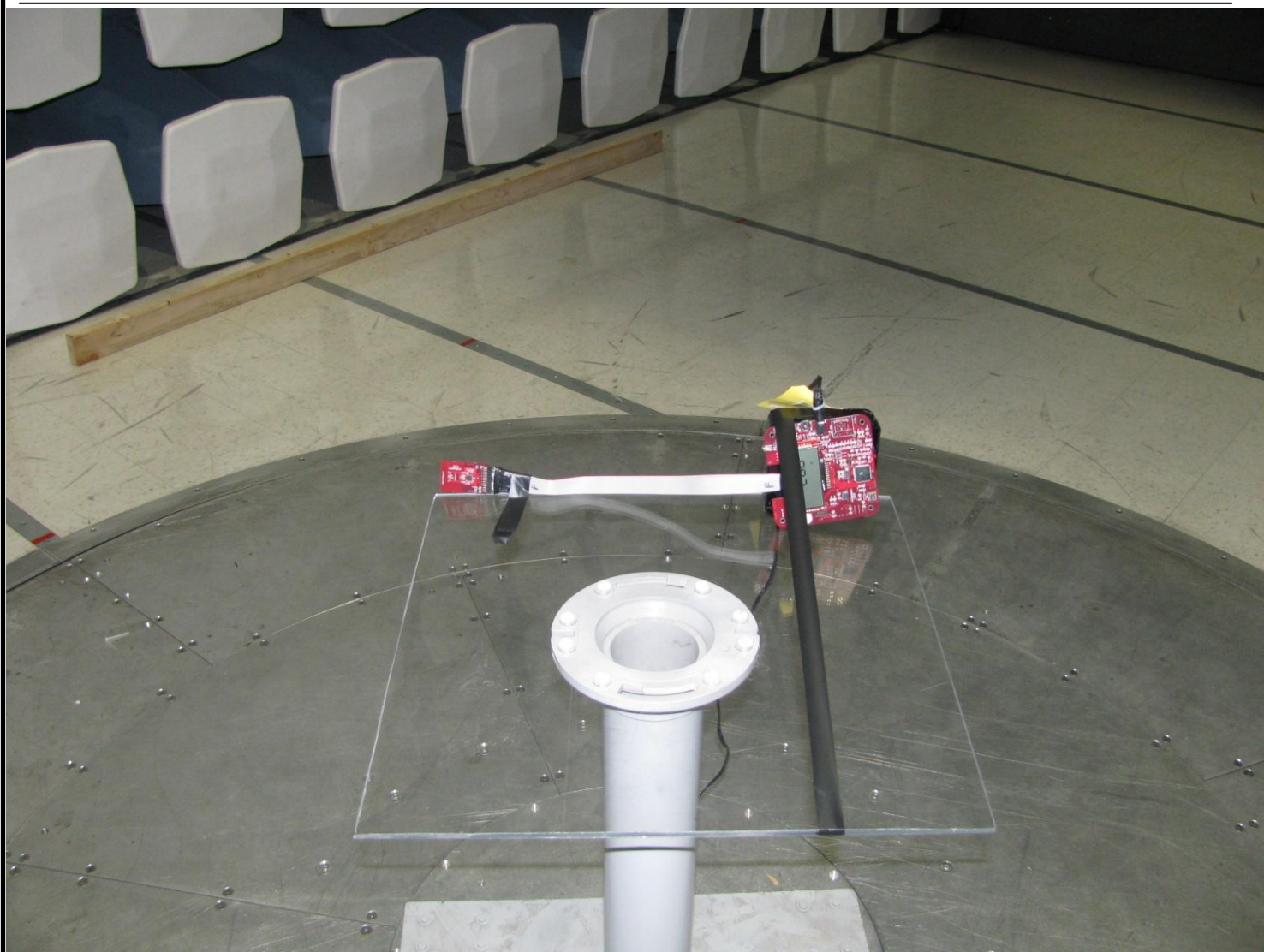
Figure 6: Setup of the Logger for Radiated Emissions Side Axis
