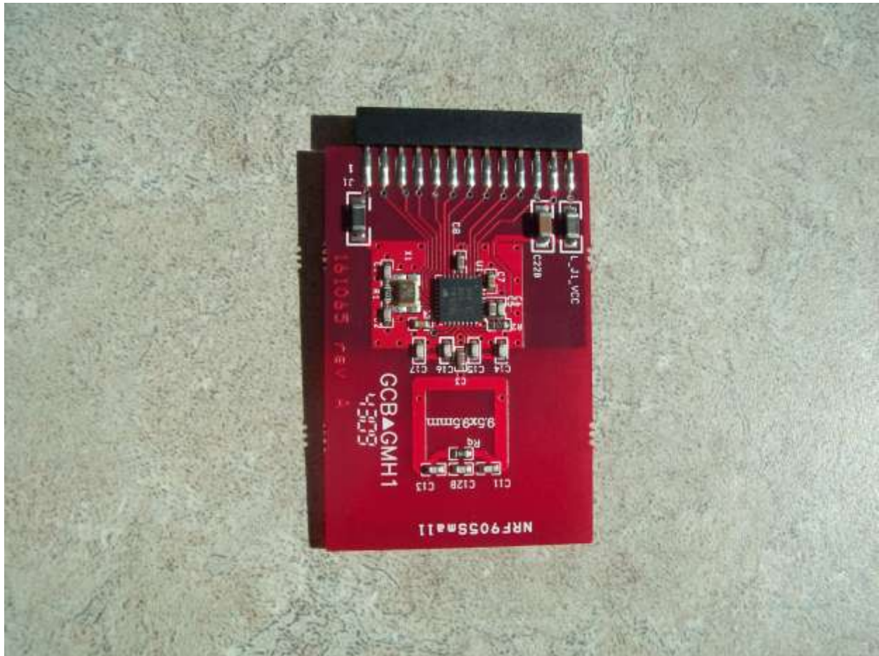
Photo 2 RF Module – Component Side
