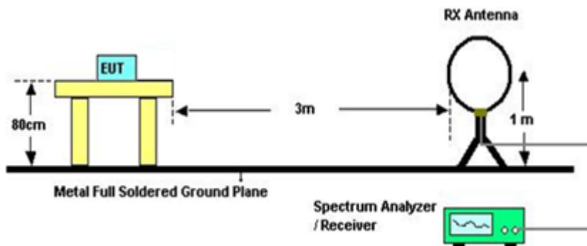
(B) Radiated Emission Test Set-Up Frequency Below 1 GHz
