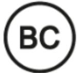
This product meets the applicable energy efficiency requirements for a battery charging system
