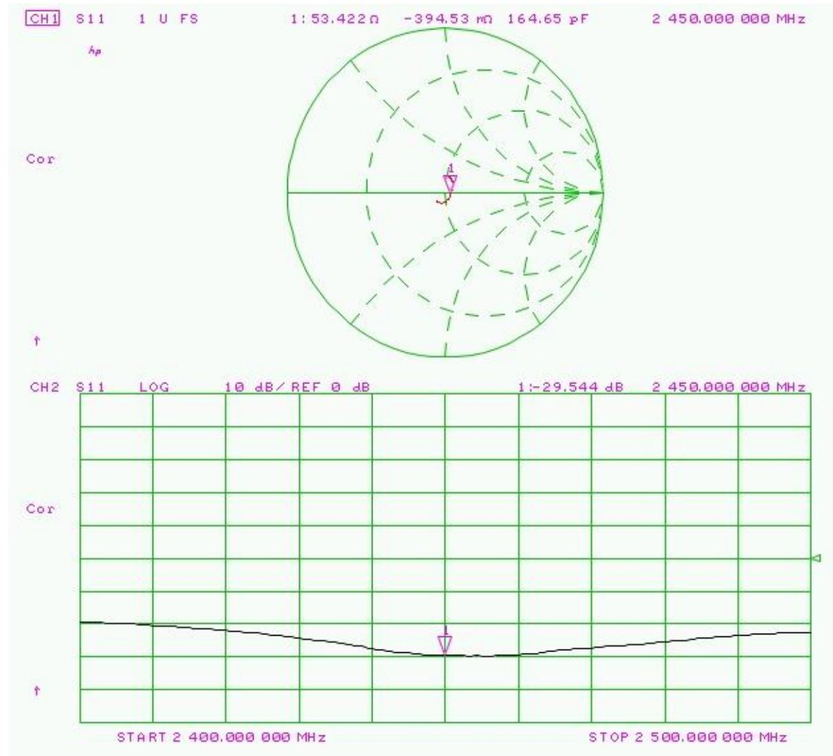
**Antenna Parameters with Body TSL**
