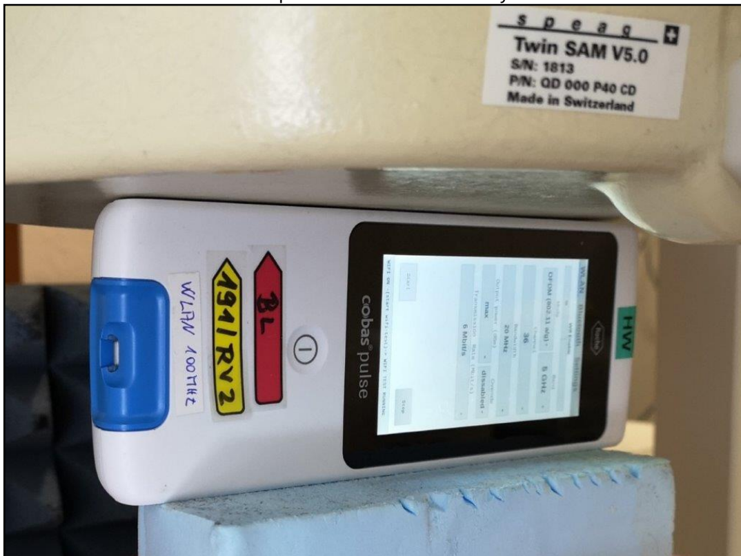
Photo 10: Test position right side without any distance
