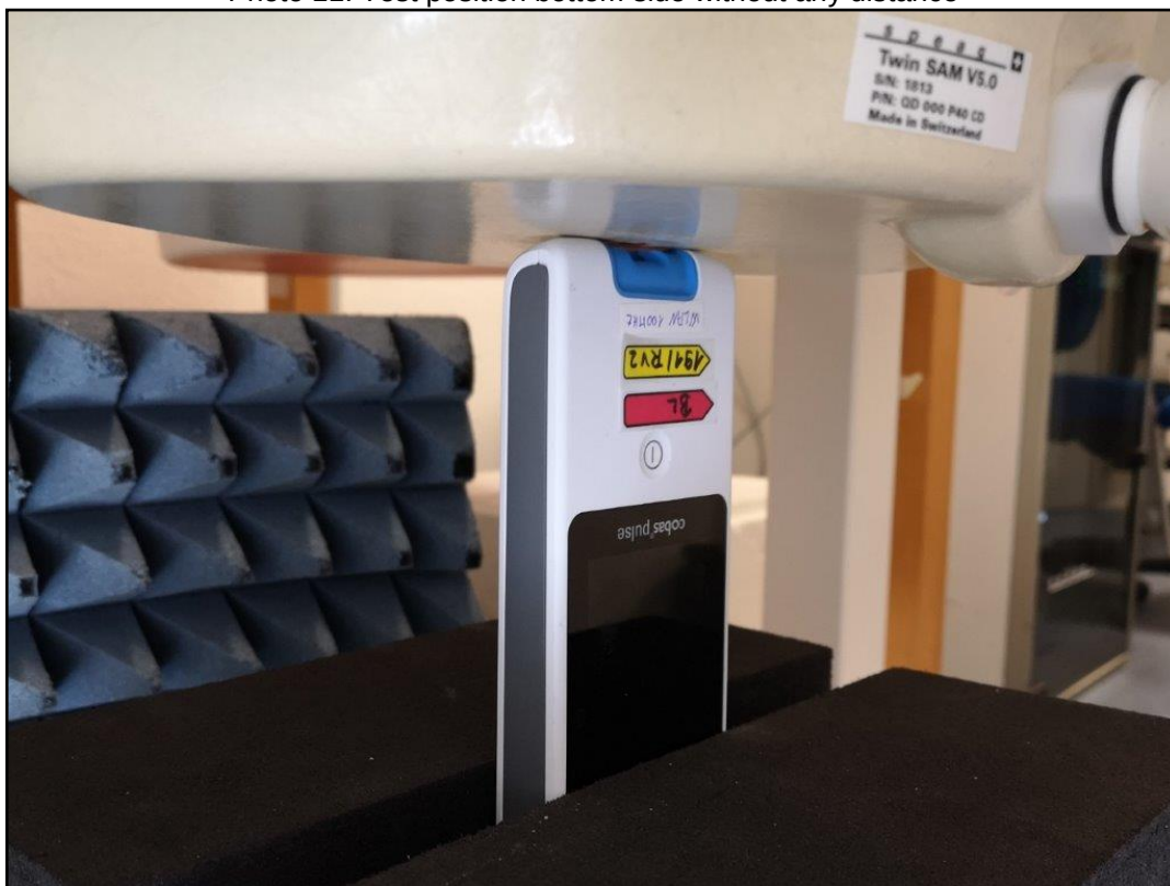
Photo 11: Test position bottom side without any distance
