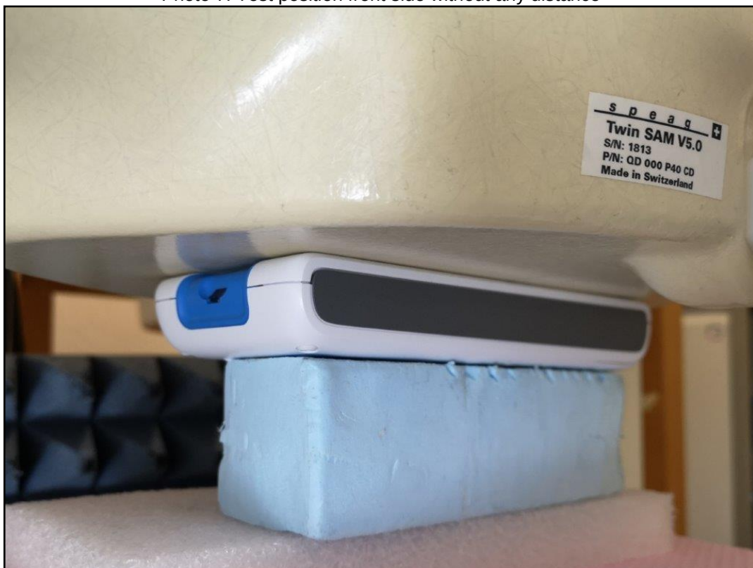
Photo 8: Test position rear side without any distance
