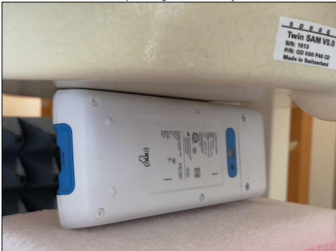
Photo 10: Test position right side without any distance
