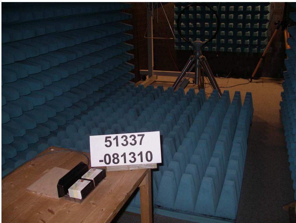
**Test setup for radiated emission measurement
