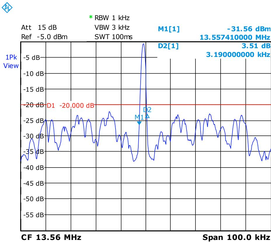
Occupied Bandwidth (-26 dB): **3.19 kHz**
