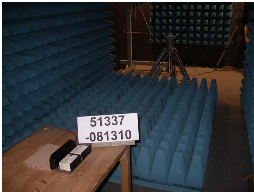
**Test setup for radiated emission measurement
