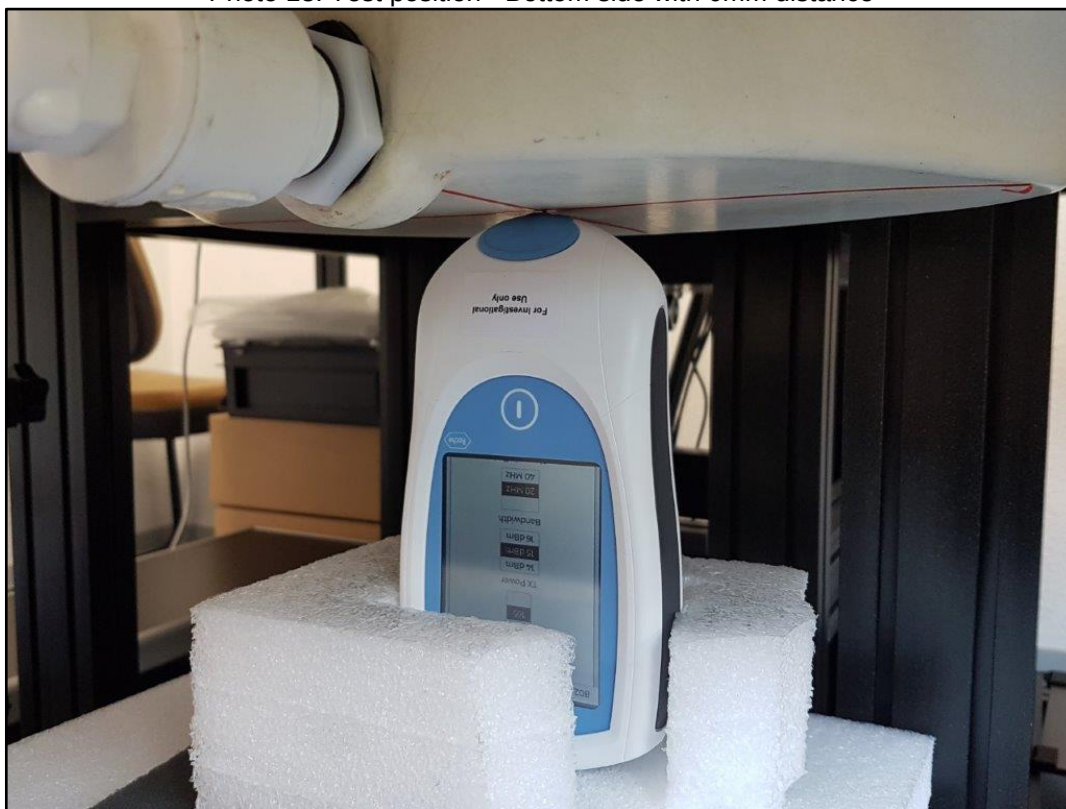
Photo 13: Test position - Bottom side with 0mm distance
