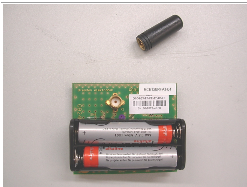
Figure 6: Back view of EUT with used \lambda/4 antenna (acc. Test report 1228-09-EE-10-PB005)
