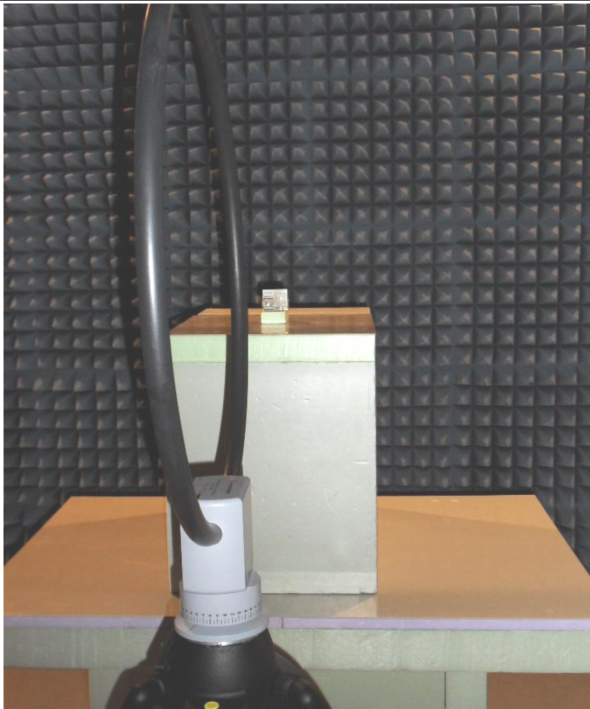
Figure 4: Measurement set-up for radiated measurement < 30 MHz acc. following sections of the report 1228-09-EE-10-PB005: 4.6
