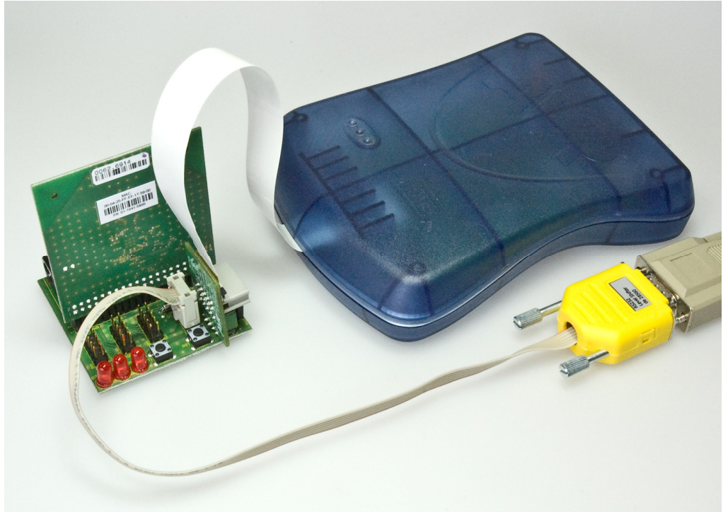
Figure 3-1. Atmel REB-CBB connected to an Atmel REB231ED with an RS232 cable plugged in and an Atmel JTAGICE mkII programming interface.
