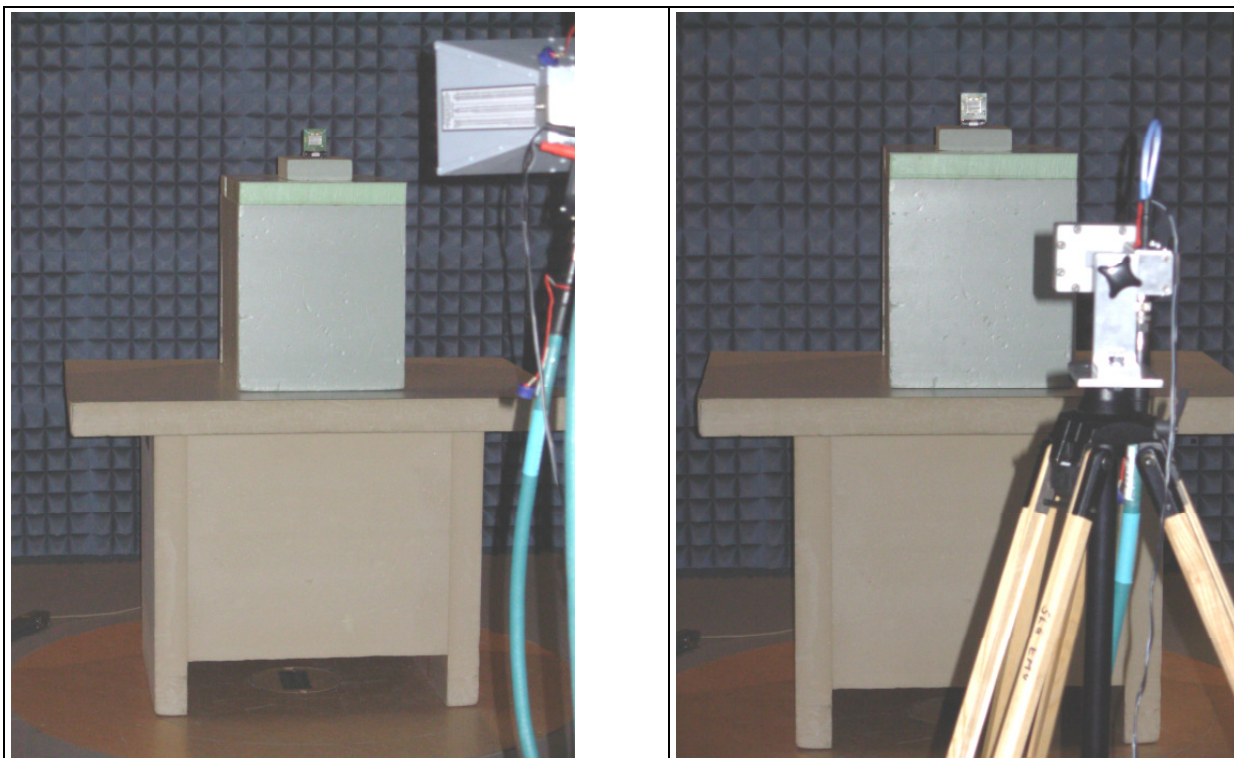
Figure 11: Measurement set-up for radiated measurement > 1 GHz acc. following sections of the report 1044-11-EE-11-PB002: 4.5.3; 4.5.4 and 4.6.2
