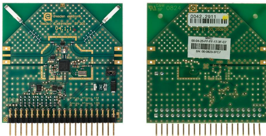
Figure 1-1. Top and bottom views of the REB231ED.
