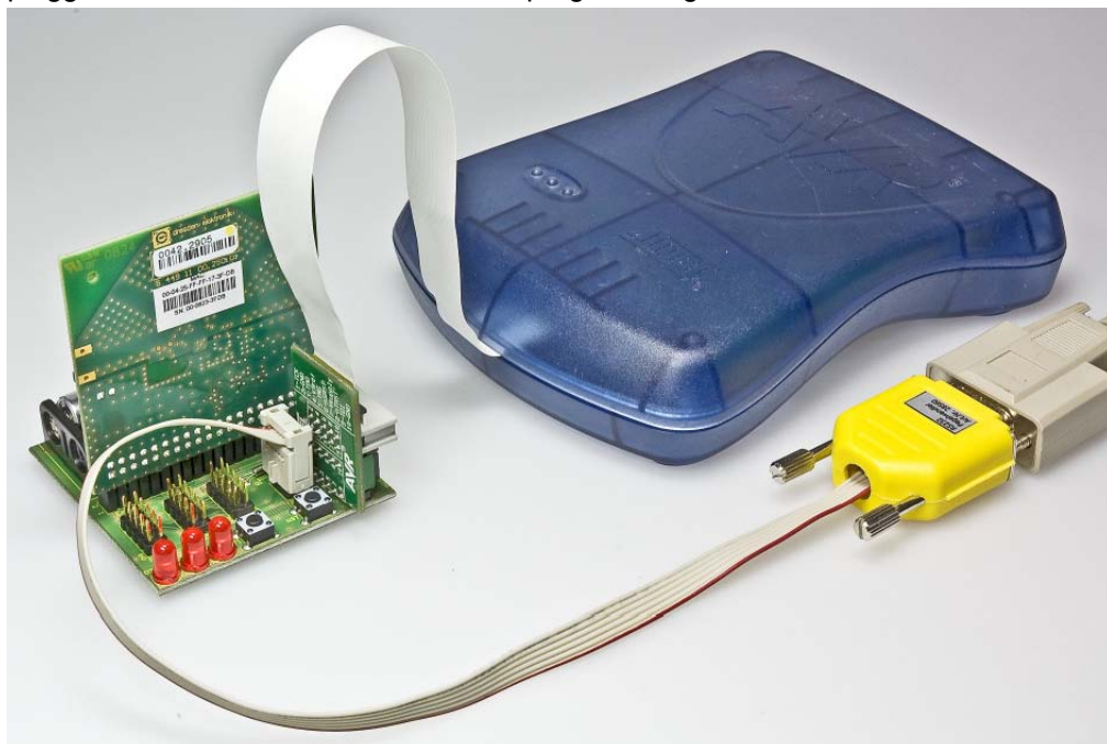
Figure 3-1. Atmel REB-CBB connected to an Atmel REB231ED with an RS232 cable plugged in and an Atmel JTAGICE mkII programming interface.
