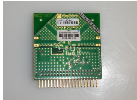
Figure 2: Bottom side of radio extension board (REB231ED)
