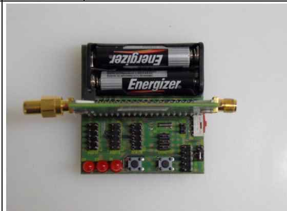
Figure 4: Top side of controller base board (CBB)
