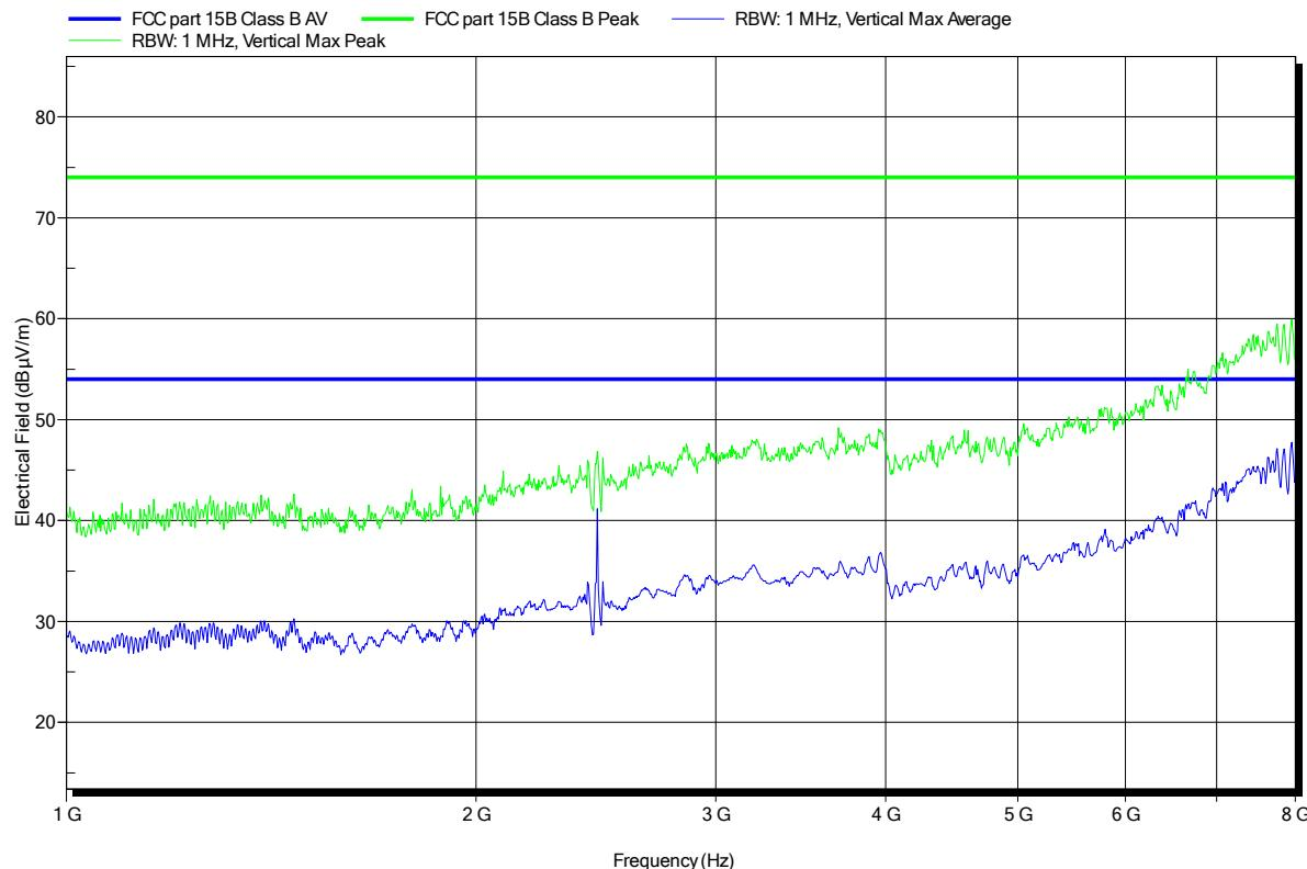
**Spurious emissions under normal conditions according to FCC Part15 B**
