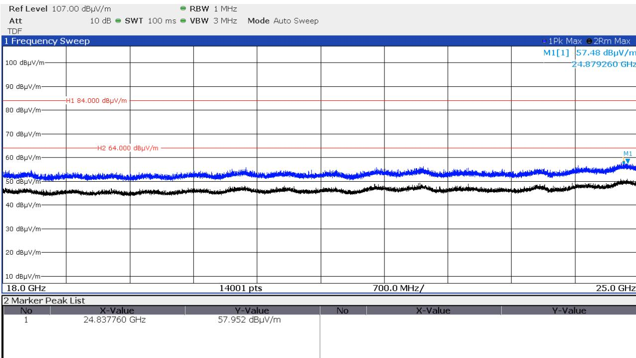
Note: the measurement distance was changed to 1 m for this frequency range, therefore the limit line has to be adjusted and was increased by 10 dB.
