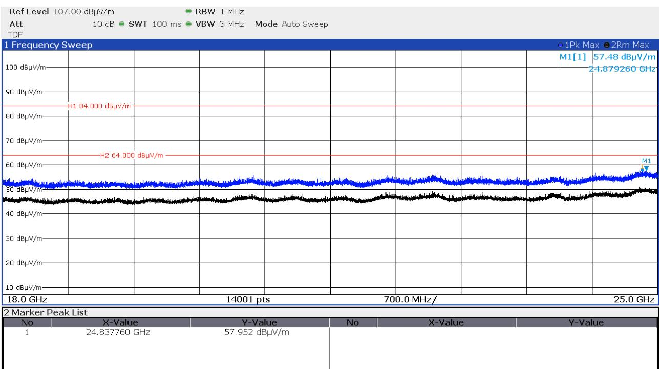
Note: the measurement distance was changed to 1 m for this frequency range, therefore the limit line has to be adjusted and was increased by 10 dB.
