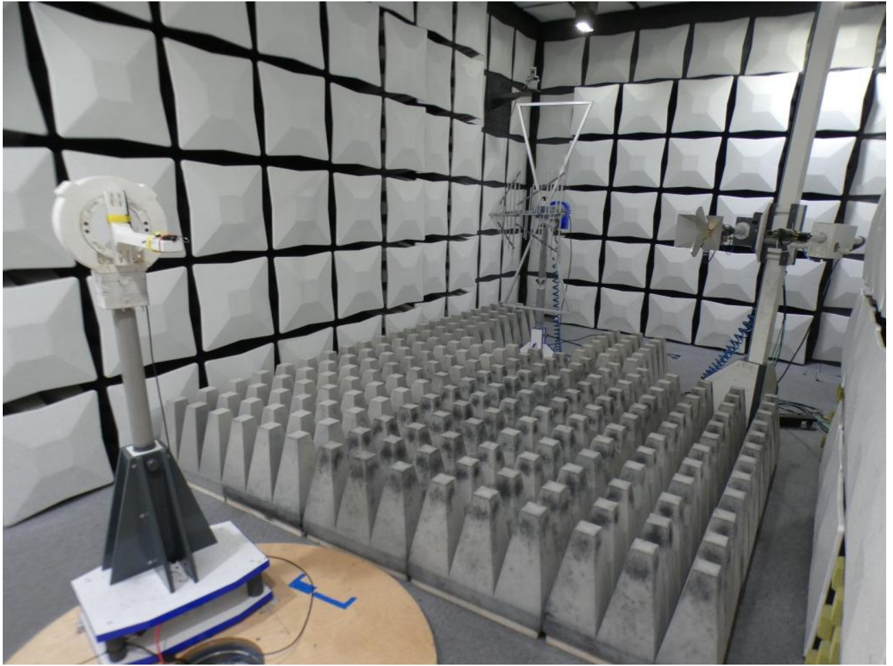
Photo 5: Test setup for radiated measurements (stand alone setup, 1 GHz - 24 GHz; FCC 15c247, ANSI 63.10)
