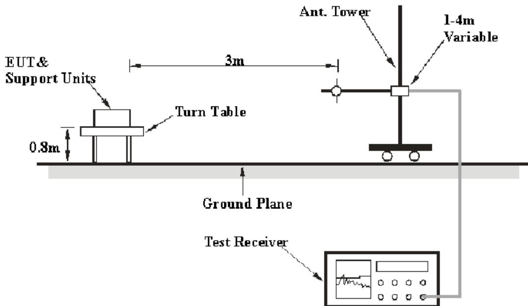
The radiated emission tests were performed in the 3 meters, using the setup accordance with the ANSI ANSI C63.4-2014. The specification used was the FCC 15.209 and FCC 15.319 limits.
