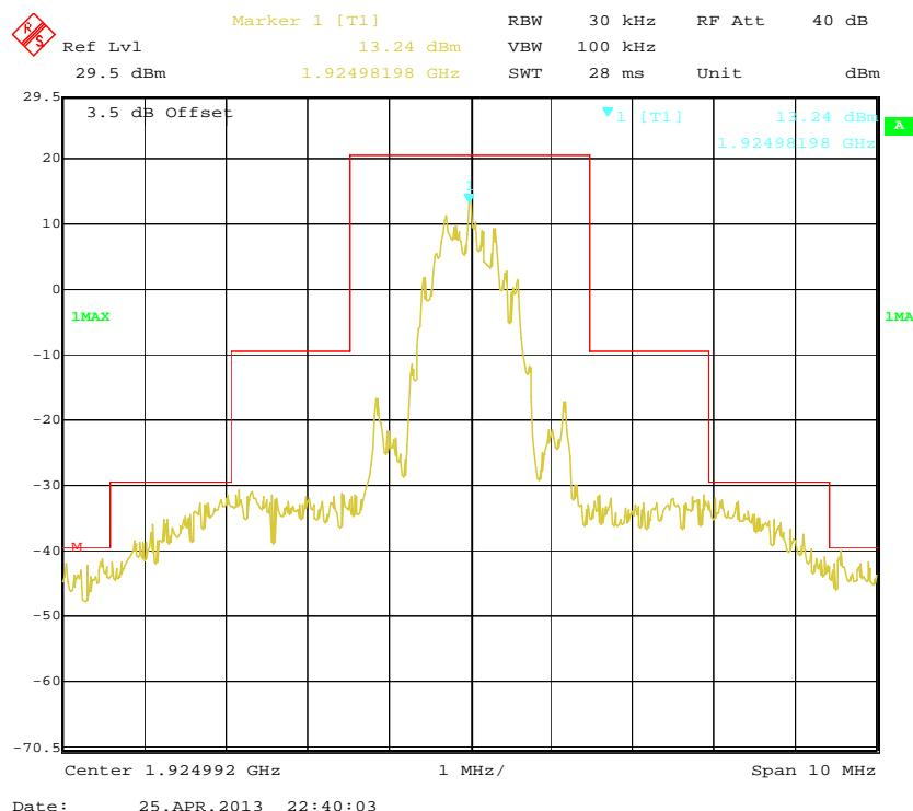
**High Channel (Unwanted Emission inside the Sub-band)**
