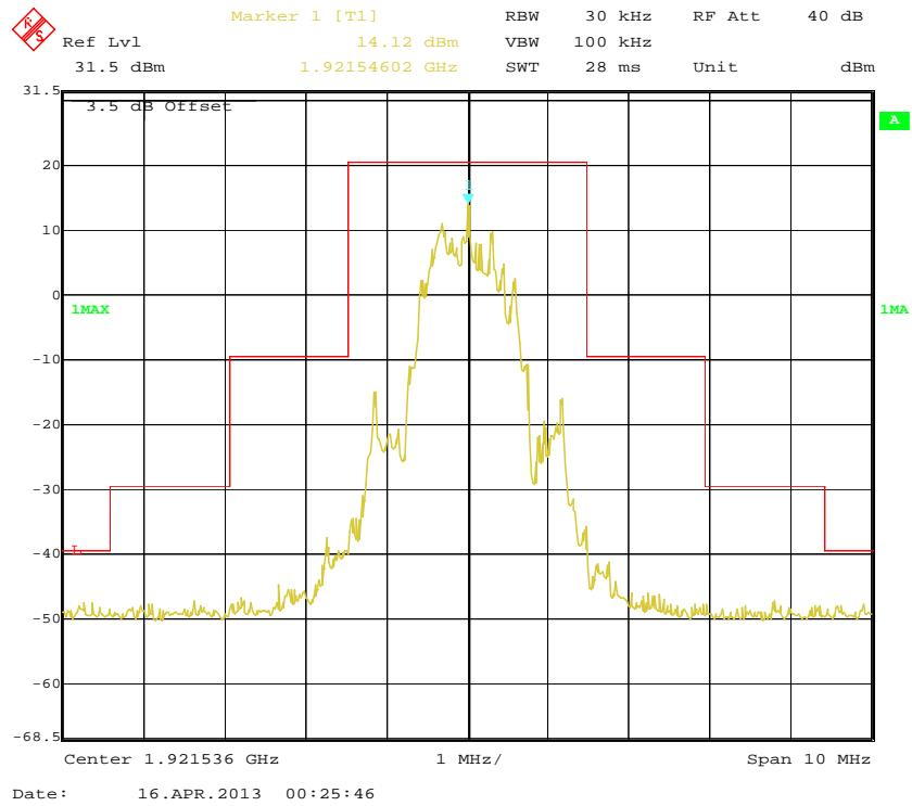
**Middle Channel (Unwanted Emission inside the Sub-band)**
