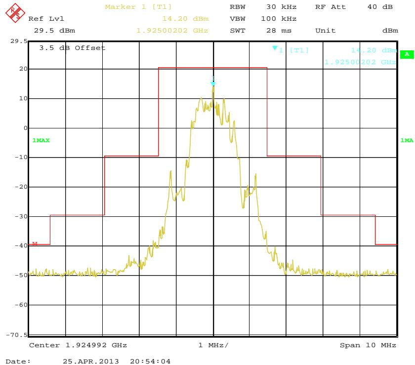
**High Channel (Unwanted Emission inside the Sub-band)**
