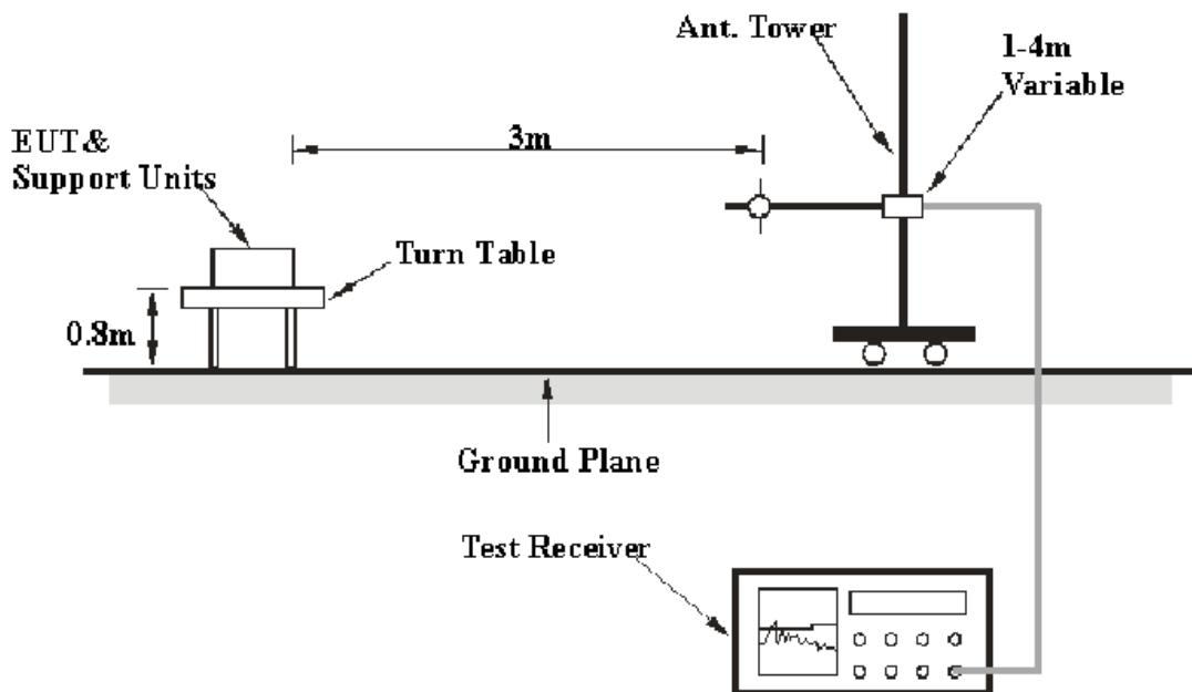
The radiated emission tests were performed in the 3 meters test site, using the setup accordance with the ANSI C63.17 - 2006. The specification used was the FCC 15§ 15.319(g).
