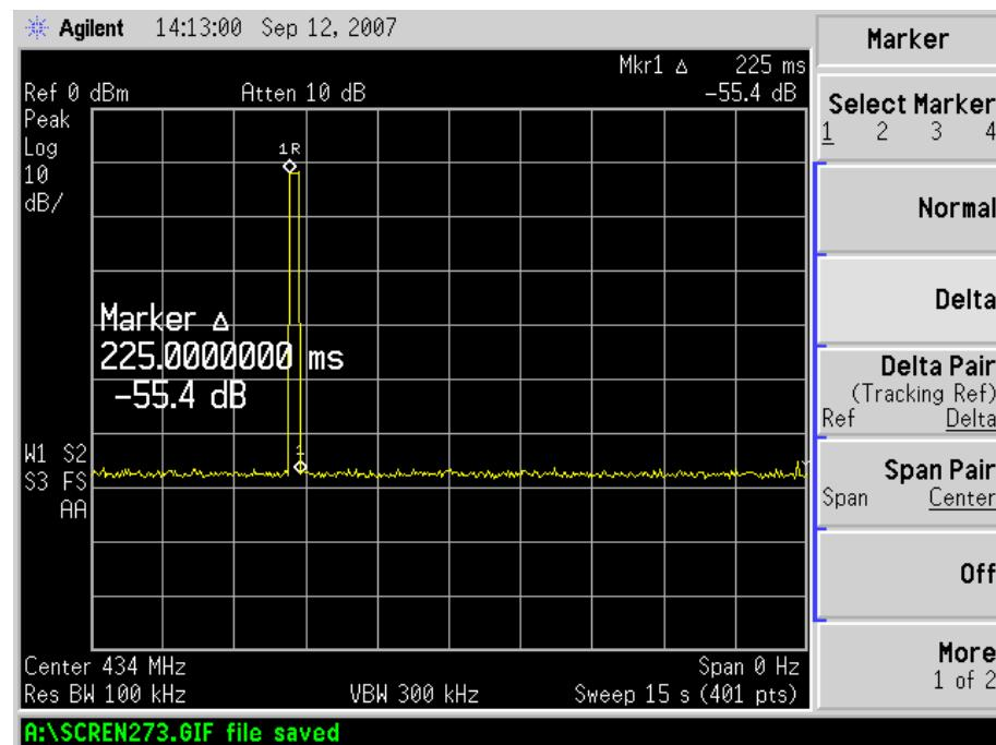
Transmitting is released even keep pressing, it is manual operation device.
