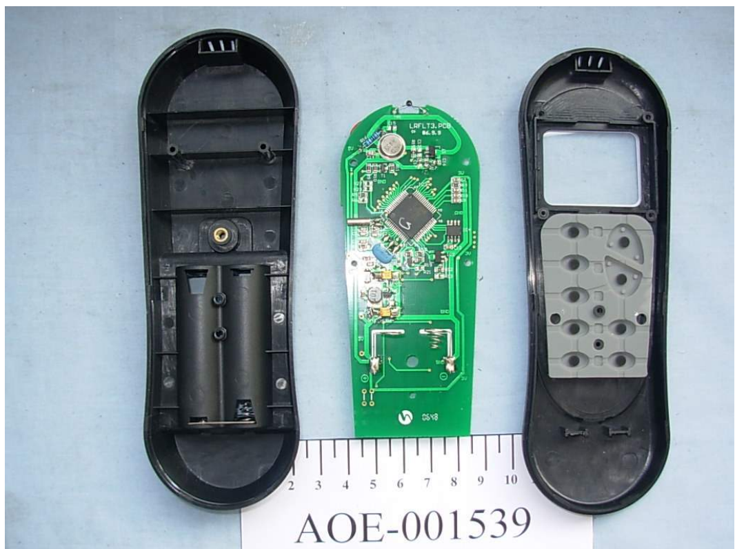
FIGURE 2 FIREPLACE REMOTE CONTROL SYSTEM (M/N: LGT202TX) COVER REMOVED
