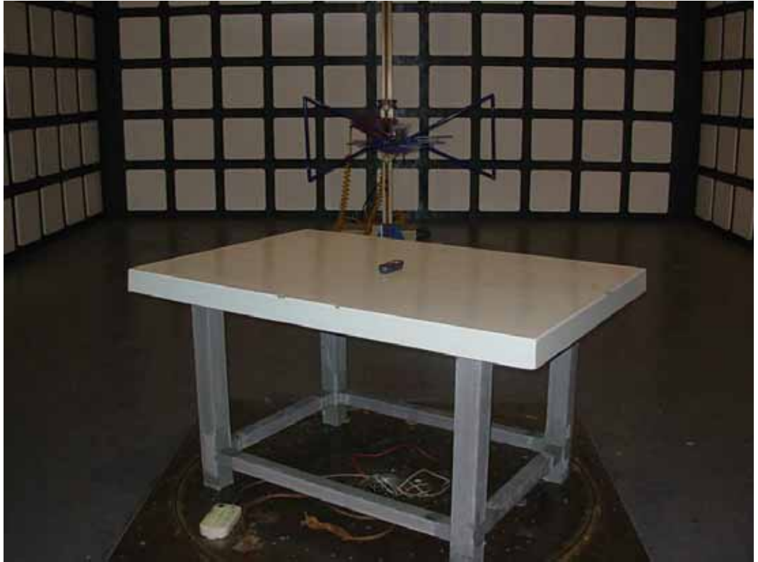
SETUP WITH MAXIMUM DETECTED EMISSION AT HORIZONTAL POLARIZATION (FOR OFF STAND TEST MODE)
