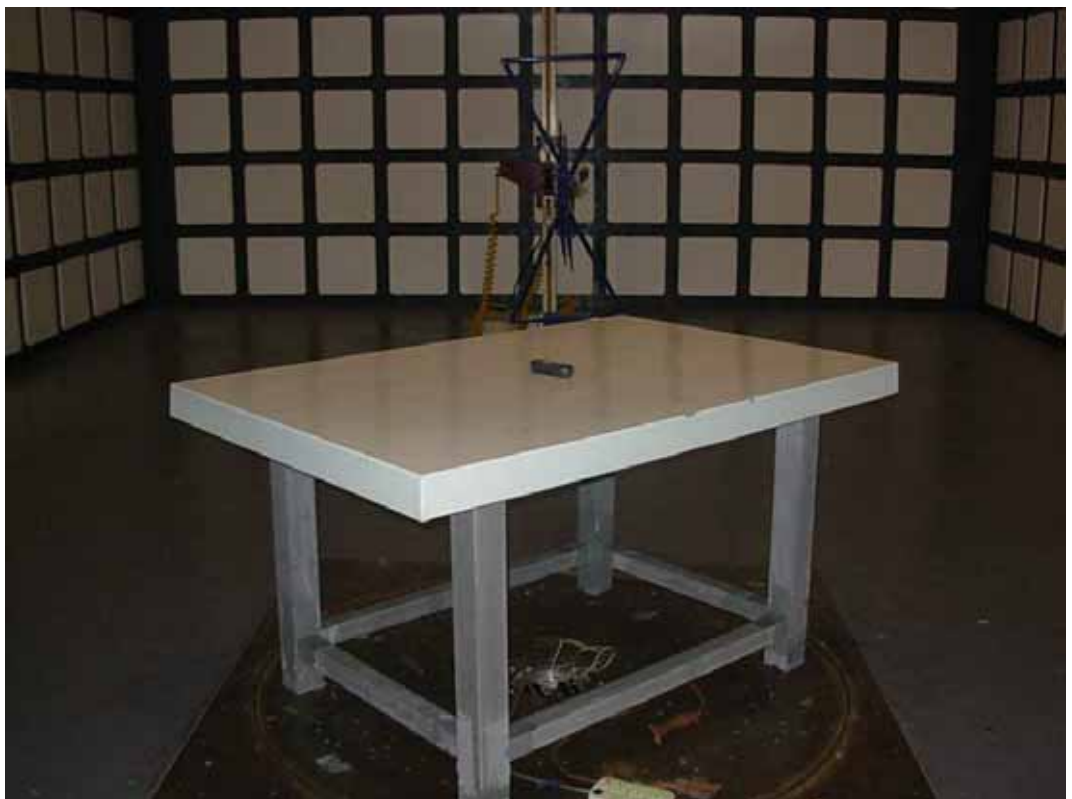
SETUP WITH MAXIMUM DETECTED EMISSION AT VERTICAL POLARIZATION (FOR OFF STAND TEST MODE)
