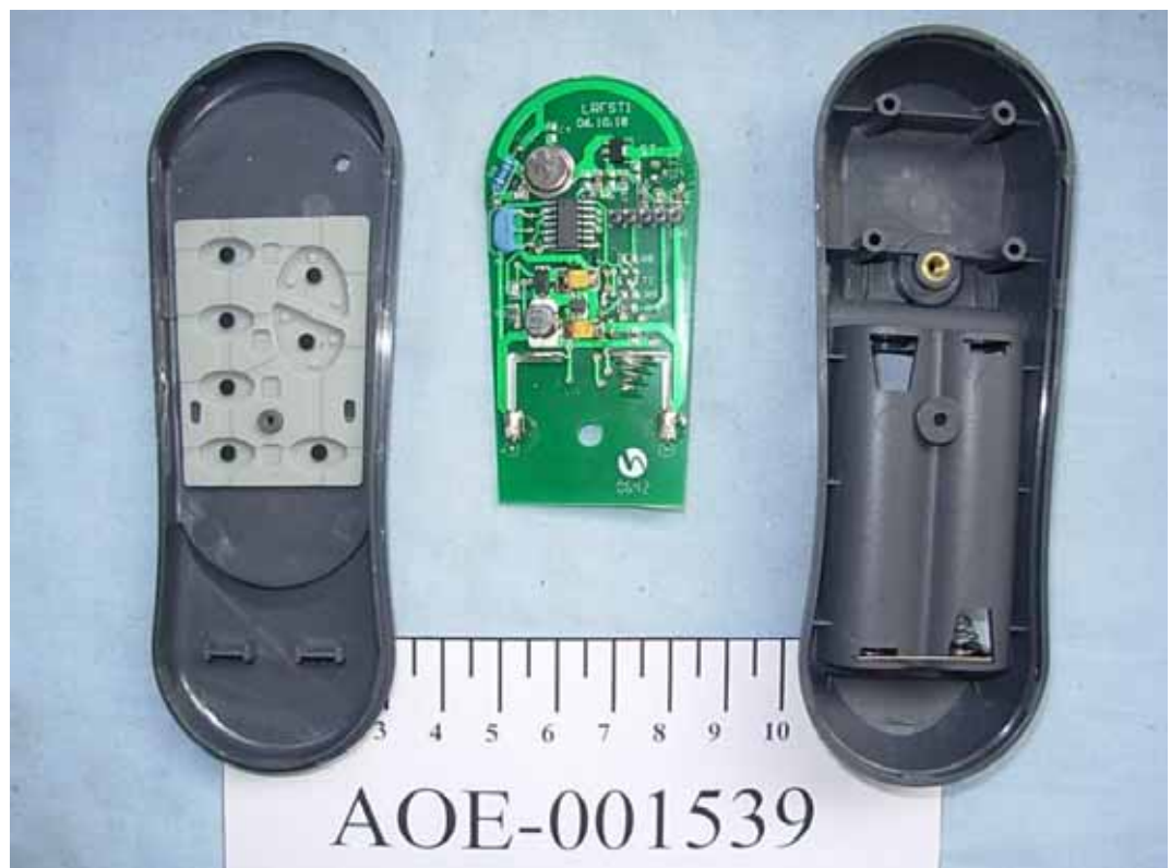
FIGURE 2 FIREPLACE REMOTE CONTROL SYSTEM (M/N: LGT201TX) COVER REMOVED
