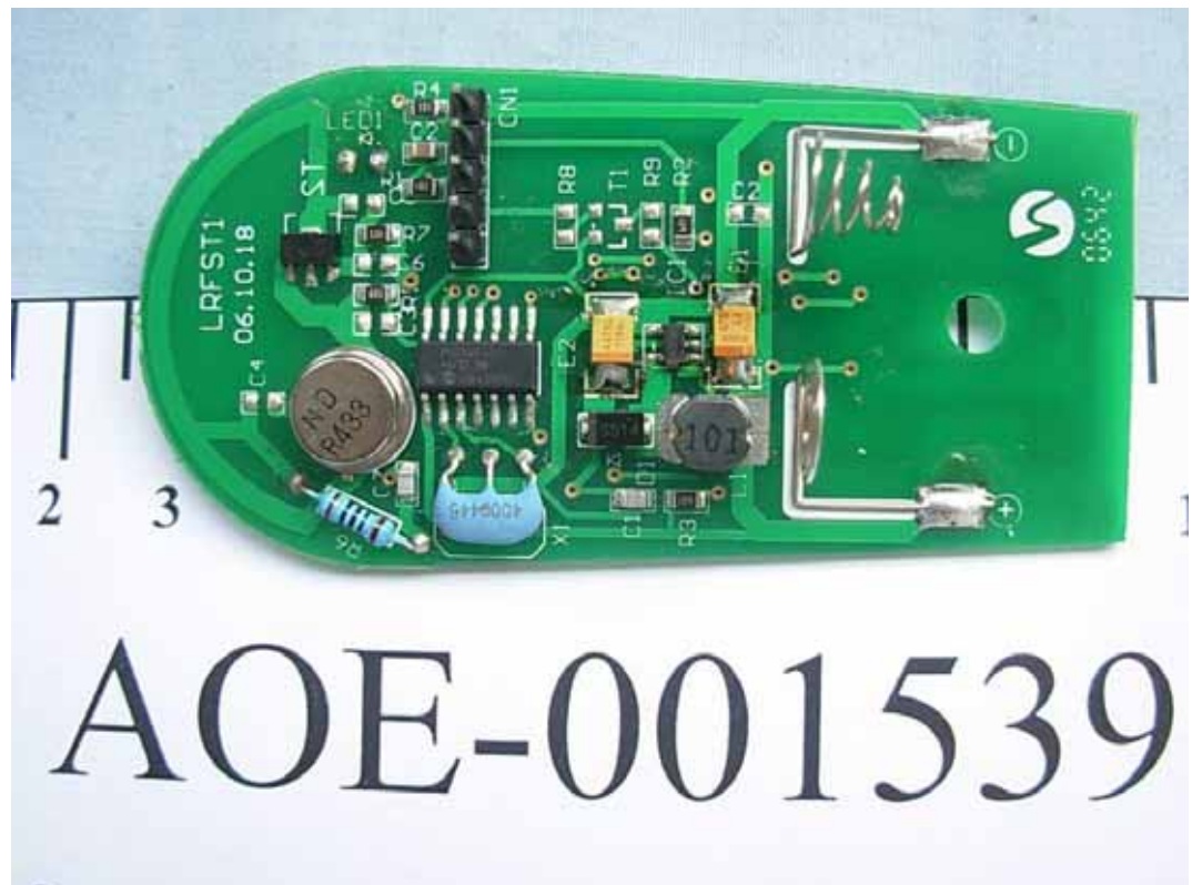
FIGURE 3 FIREPLACE REMOTE CONTROL SYSTEM (M/N: LGT201TX) MAIN BOARD (SOLDERED SIDE) MAIN BOARD (COMPONENT SIDE)
