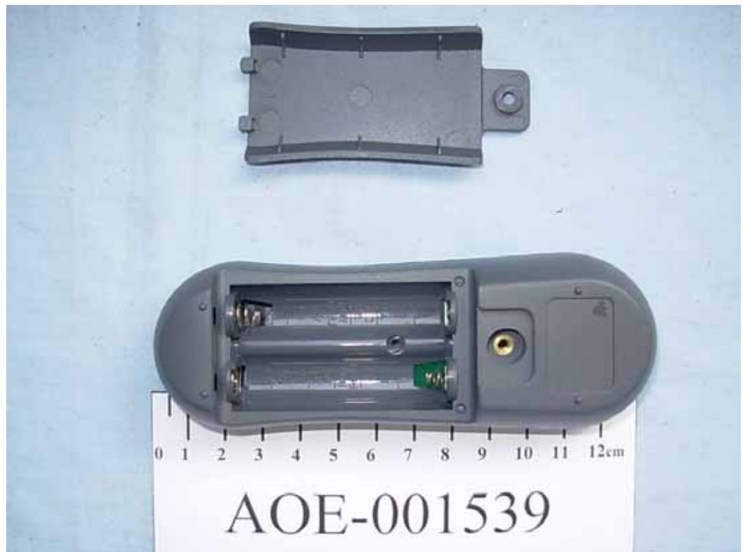
FIGURE 1 FIREPLACE REMOTE CONTROL SYSTEM (M/N: LGT201TX) BATTERY COVER REMOVED
