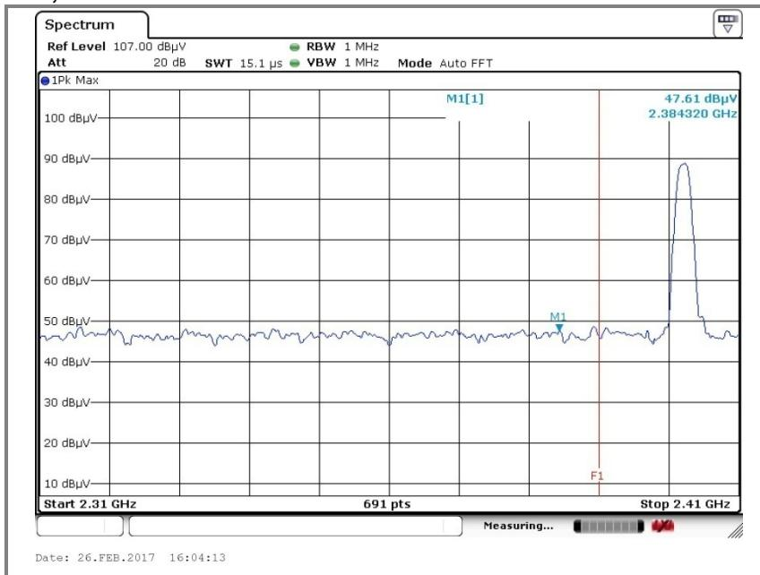
**B. High channel(2 480 MHz) 2 483.5 – 2 500 MHz measurement**
