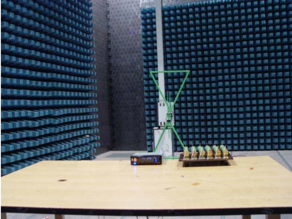
Photo 1 Radiated Emission Test
