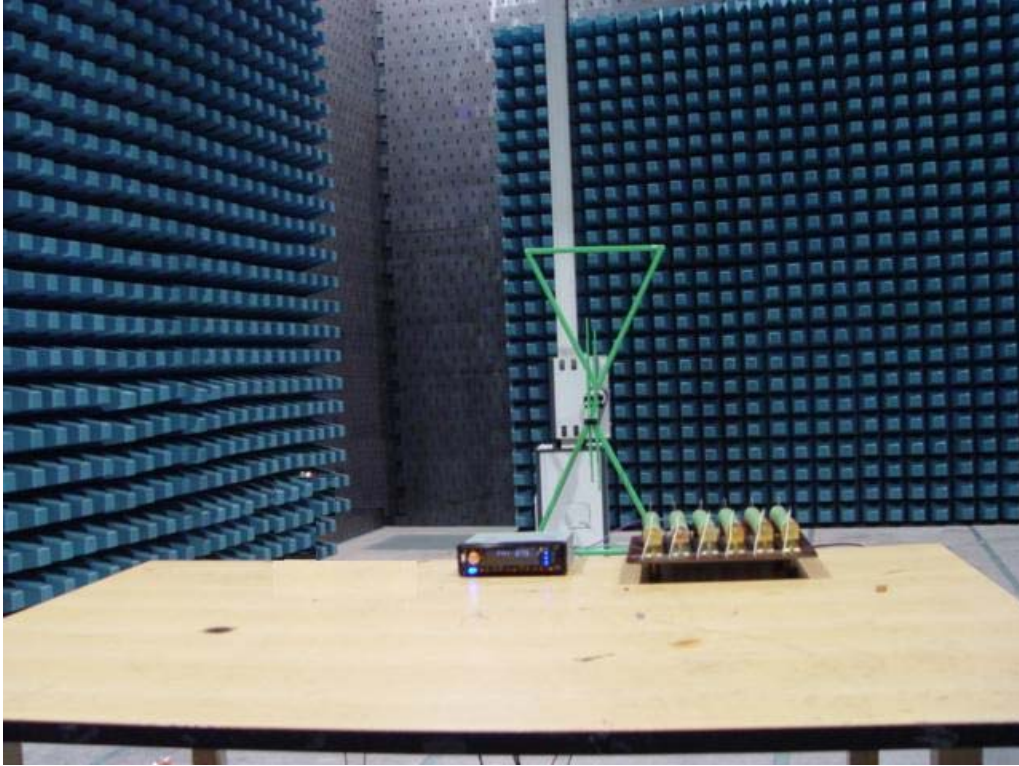
Photo 1 Radiated Emission Test
