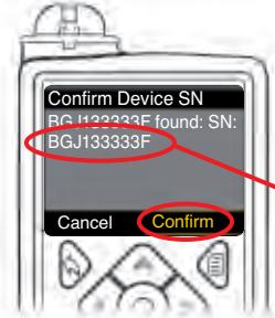
12. Check that the SN (serial number) on the **pump** screen matches the **meter** SN on the **meter** screen. If they match, scroll to **Confirm** on the pump. Press Select button
