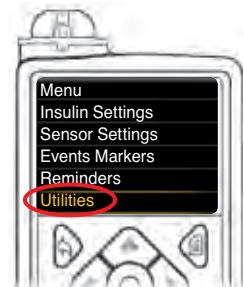
6. Pick up your pump. Press any button to turn the screen on, then press the **Menu** button . Use the down arrow to scroll to **Utilities**. Press Select button .
