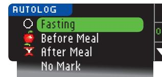
After you apply blood to the test strip, use the ▼ to select **Fasting**, **Before Meal**, **After Meal**, or **No Mark**, and then press **OK**. (Scroll down to see **No Mark**.)
