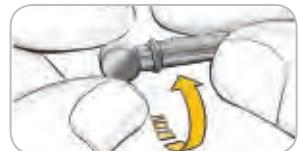
2. Loosen the round protective cap on a lancet by rotating it 1/4 turn, but do not remove it.
