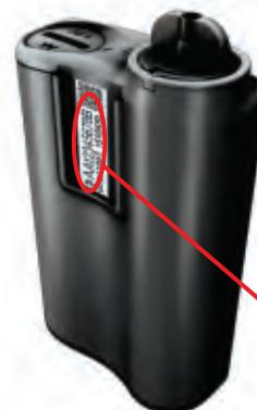
14. Turn the pump over. Check that the SN on the back of the **pump** matches the **pump** serial number now on the **meter** screen.
