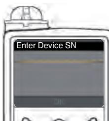
10. Pick up the pump. Enter the meter serial number (SN) shown on the meter into the pump screen. Use the up and down buttons to select the characters, then press the right button to move to the next character. Keep pressing up to get to the alphabet. Press down to go in reverse (starting with "Z"). Press the Select button after entering the last SN character. Select **OK** on your pump.
