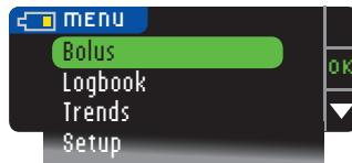
As the battery is used, the battery symbol on the screen gradually shows less fill colour. The colour of the battery fill turns yellow when the battery is low and then red when your battery is almost out of charge.
