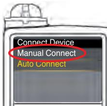
9. Place the meter and pump next to each other. Select **Manual Connect** on your pump. Select **Manual Connect** on your meter.
