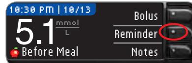
1. With the test strip still in the meter, press **Reminder**.
