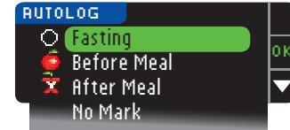
9. If you have the AutoLog feature turned ON, the AutoLog screen appears. Select **Fasting**, **Before Meal**, **After Meal**, or **No Mark** by pressing the **OK** button when your selection is highlighted. Scroll down to see **No Mark**.
