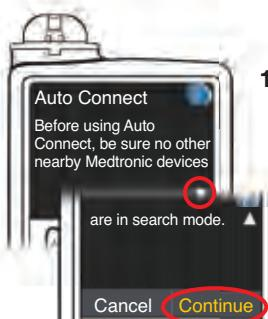
11. Read pump screen. Be sure other nearby Medtronic devices are NOT in search mode. Use the down arrow to scroll to the next page. Use arrow buttons to scroll to **Continue**. Press Select button .
