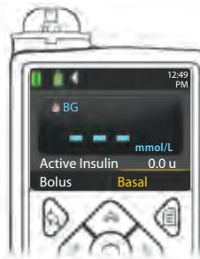
16. Hold the back button on the pump until you see the home screen. Put down the pump and pick up the meter.
