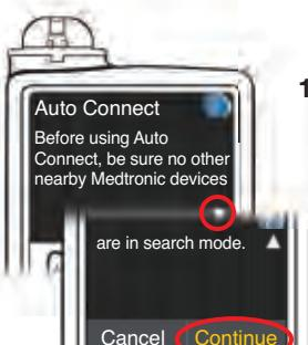
10. Read the pump screen. Be sure other nearby Medtronic devices are NOT in search mode. Use the down arrow to scroll to the next page. Use arrow buttons to scroll to **Continue**. Press Select button .
