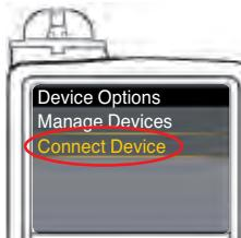
8. In the Device Options menu, scroll to **Connect Device**. Press Select button .
