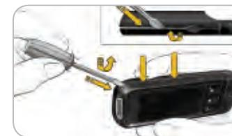
To remove the battery for proper disposal, you will need to pry the upper and lower cases apart.
